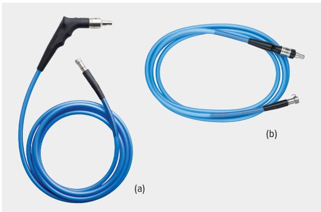
Light guides are made from hundreds of high-quality fibers. Instead of gluing fibers, we fuse ours at the proximal end to maximize light transmission. The unique handle increases durability and prevents accidental removal of the light guide. Additionally, our transparent casing makes it easier to monitor when to replace light guides.
