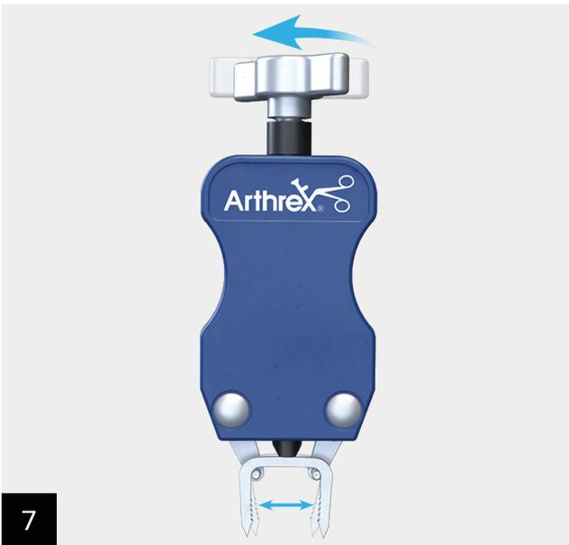
Turn the knob on the DynaNite delivery device clockwise until the staple legs are open to a width equal to the predrilled holes.
